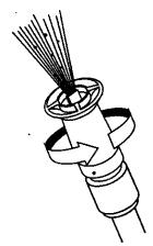
Twist nozzle counterclockwise for "fan" pattern.
