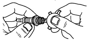
Install spark plug, tighten securely.
