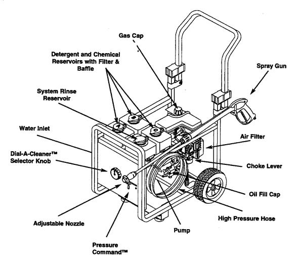
Adjustable Nozzle - Adjust for high or low pressure; narrow or fan spray.
