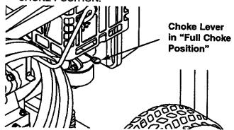
Note: If restarting a warm engine after a short shutdown, move choke lever to "NO CHOKE POSITION."
